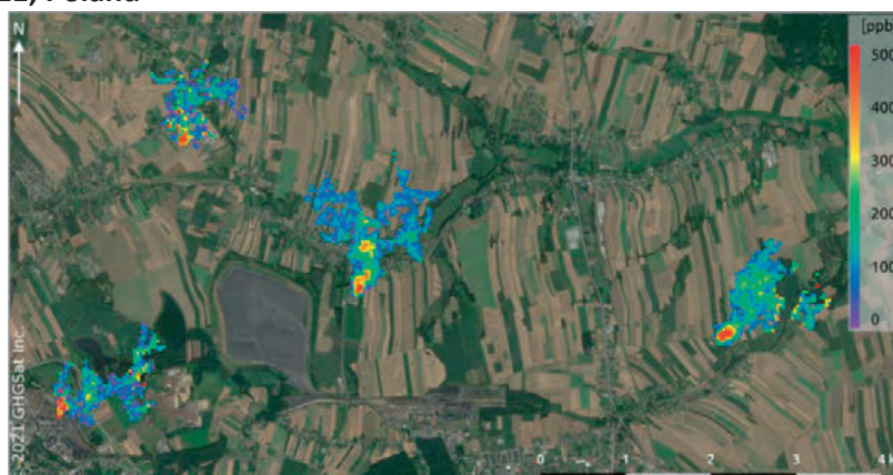
Methane concentrations above atmospheric background from four working coal mine vents, March 31, 2021, Poland
